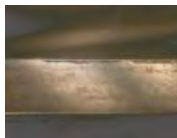
Relief face Flank wear 0.09 mm
