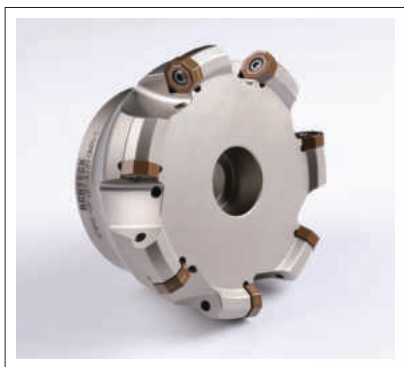
AFM40-ON05-C-45, with 45 degree approach angle, using 16 cutting edge insert with wiper edge. Used in finish milling the flange face of turbocharger casing
